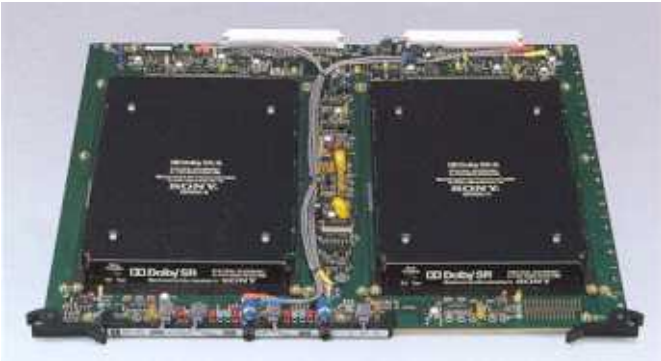
BKH-3080 Audio Processor Board A one board, plug-in type audio processor for the BVH-3000/3100, which offers a high quality noise reduction system (Dolby A/Dolby SR).
